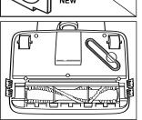
Reassemble the belt and the baseplate and check bristle height above baseplate at each end of brush.
